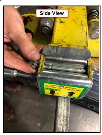
Carefully remove the tension / shear pin:
